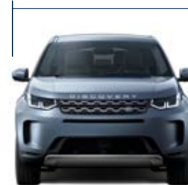
Width 2,069mm mirrors folded Width 2,173mm mirrors out
